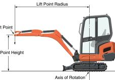
\*The lifting capacities are based on ISO 10567 and do not exceed 75% of the static tilt load of the machine or 87% of the hydraulic lifting capacities of the machine. \*\*The excavator bucket, hook, sling and other lifting accessories are not included on this table.
